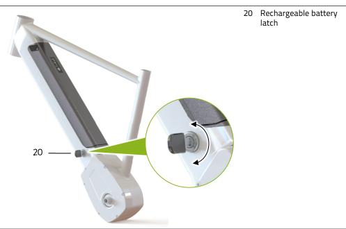
The various assembly variants of the rechargeable battery require various rechargeable battery latch designs. You can obtain detailed information about locking
