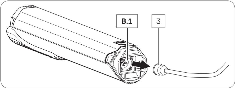
3. Then disconnect the power cord from the AC adapter and keep the two parts of the charger separate from each other.
