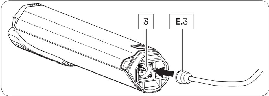
2. Plug the power plug into a suitable wall outlet to establish the power connection.
