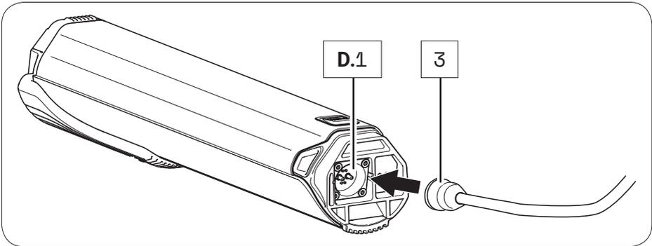
2. Plug the power plug into a suitable wall outlet to establish the power connection.
