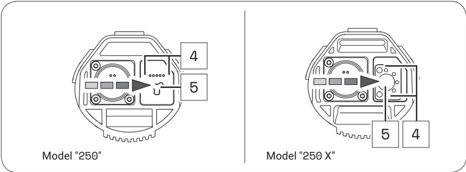
If none of the LEDs on the charge indicator light up after pressing the On/Off button, this indicates that the battery is damaged.
