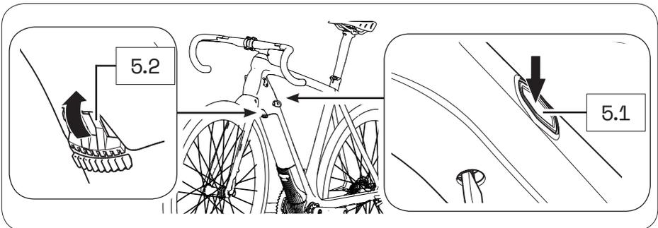
3. Press and hold down the push button and carefully lower the drivepack out of its holder in the down tube.
