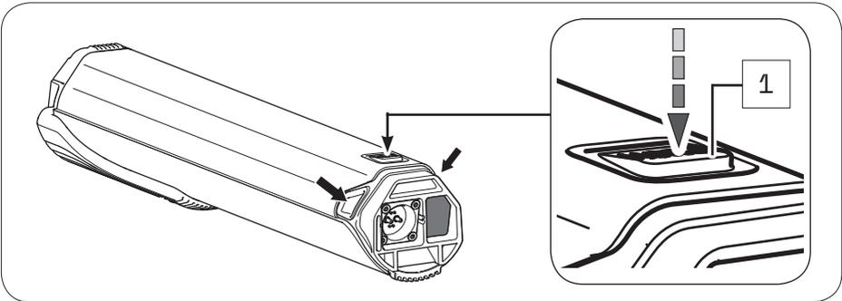
3. Press and hold the push button, grasp the battery on the two handles and gently pull the battery out of the battery holder. The two handles are located at the side of the upper battery end (see arrows).
