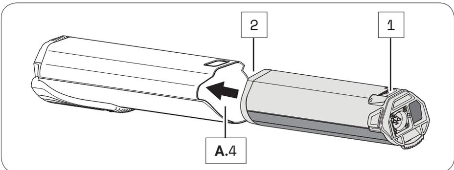
The battery is designed so that it can only be inserted into the battery receptacle when correctly aligned.
