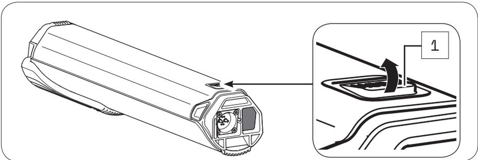
If the battery does not lock, pull it out again if necessary, make sure that there is no dirt inside the drivepack to obstruct insertion, and then try inserting the battery again. Do not use the drive system if the battery cannot be locked, but contact an authorized specialist.
