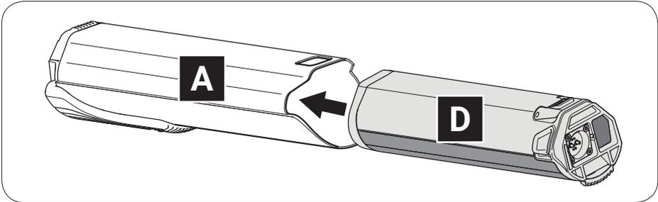
4. Carefully insert the battery as far as possible into the battery holder. The battery is automatically locked when you have inserted it correctly. If the battery does not lock, repeat the procedure. Do not use the drive system if the battery cannot be locked.
